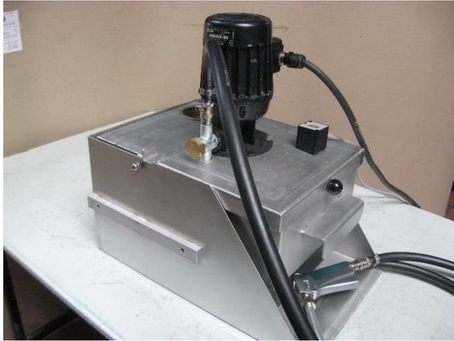
With its efficient mixing system and a tank which is specially designed to avoid sedimentation, this is an essential accessory for all magnetic particle inspection equipment.
